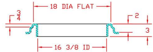
FILLWELL DETAIL 1/8 SCALE
